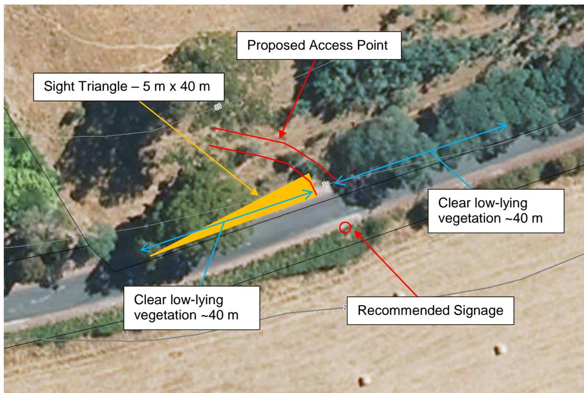
**Figure 6 Recommended Access Works**
