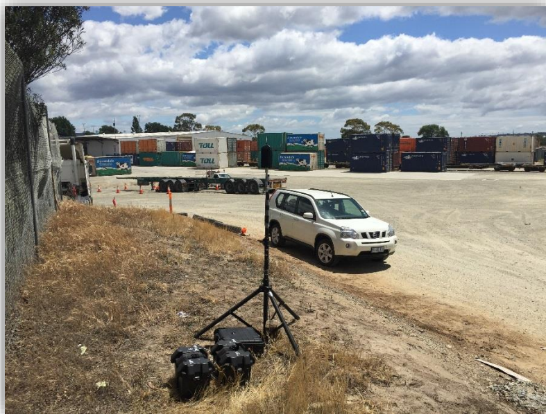
Figure 4 – Sound level meter at unobserved measurement position, view to the north-west.
