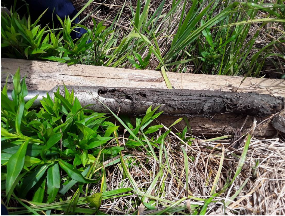
Soil composition inside flood wall (BH_B)
