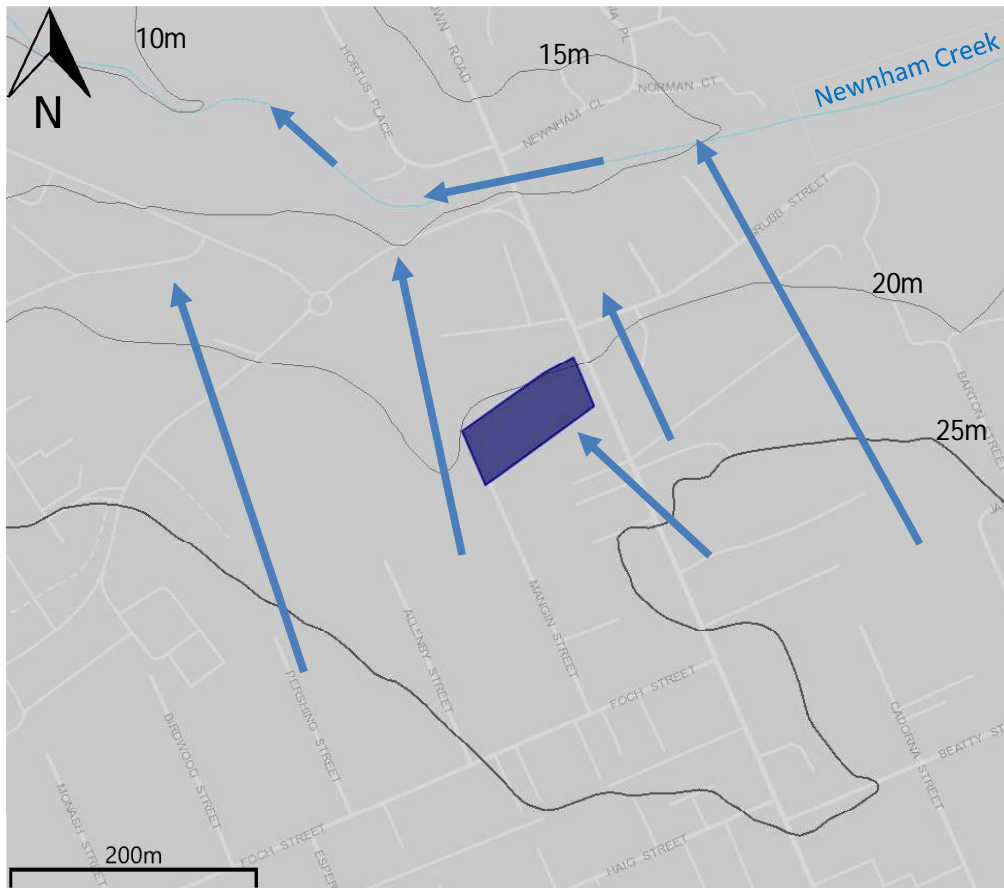
Figure 4: Inferred Groundwater Flow Direction showing AHD contours
