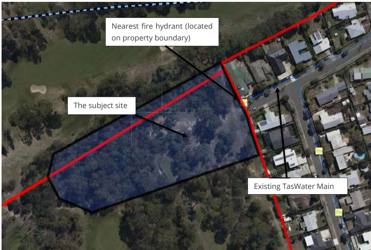
Figure 3 – Area of subject site being subdivided. Blue lines represent water mains and yellow FH squares represent fire hydrants. (source: The LISTMap)
