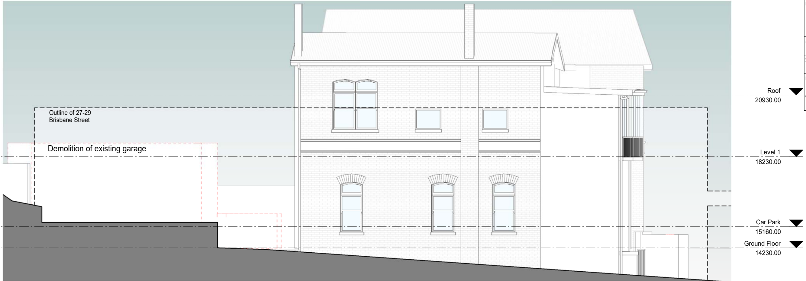
2 Existing North East Elevation 1 : 100
