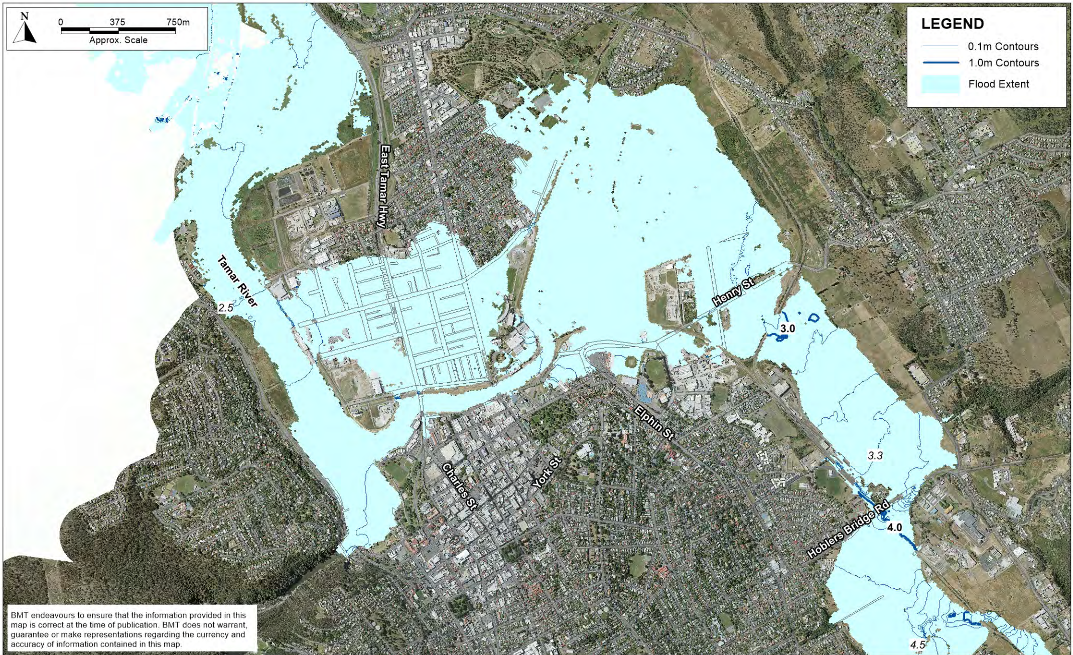
Figure C-1 No Levee Scenario Mapping 20% AEP Event Flood Level
