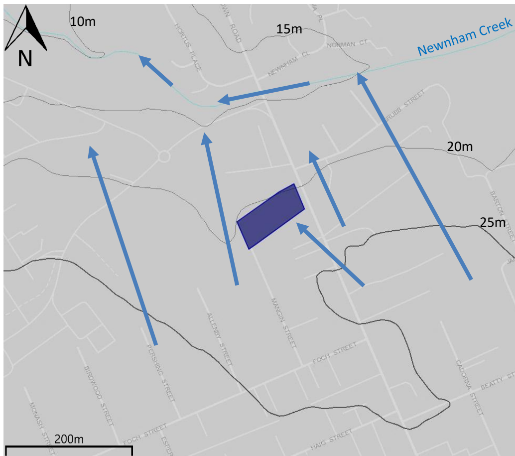
Figure 4: Inferred Groundwater Flow Direction showing AHD contours
