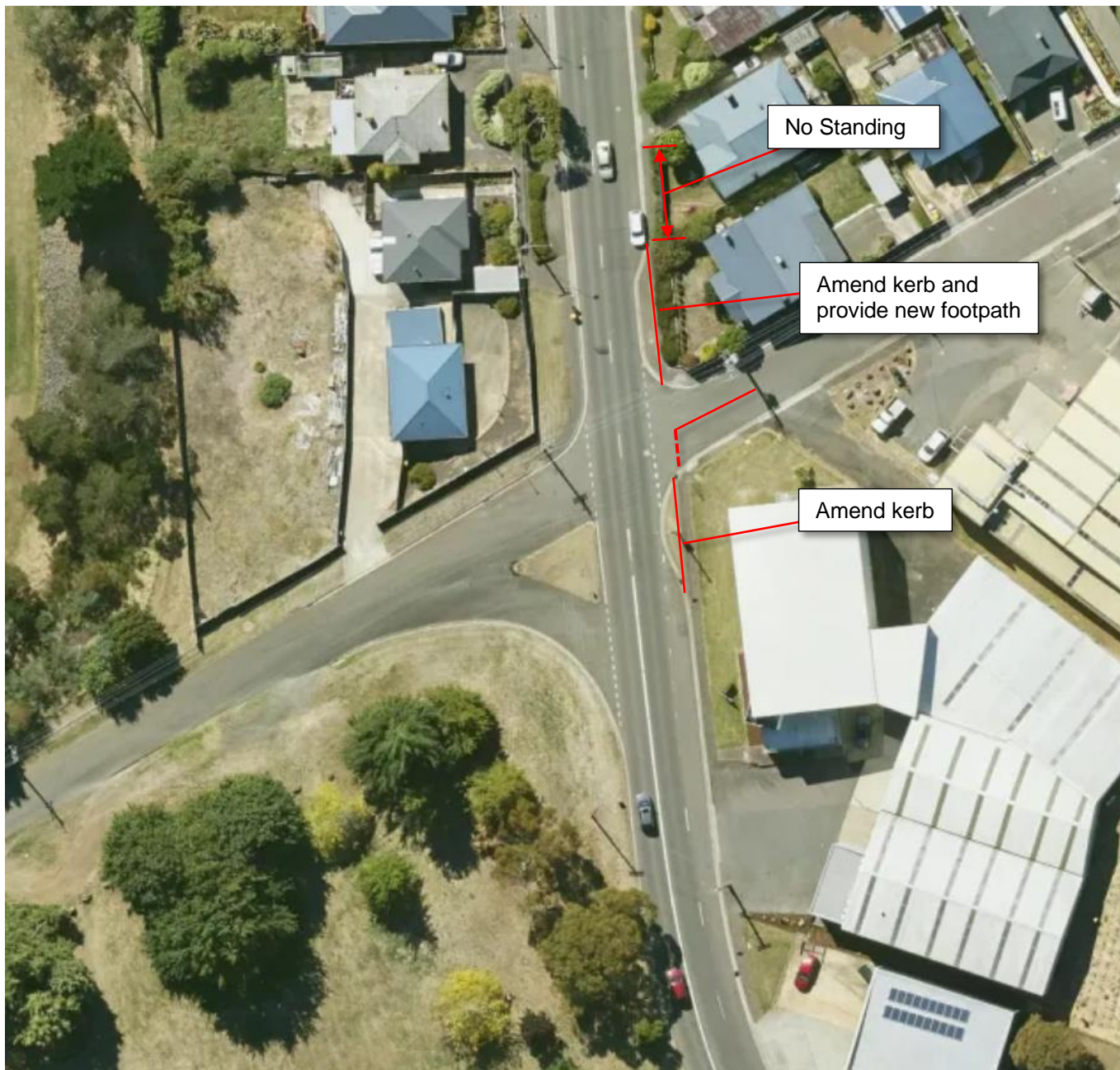
Figure 8 Westbury Road / Rose Lane right turn treatment
