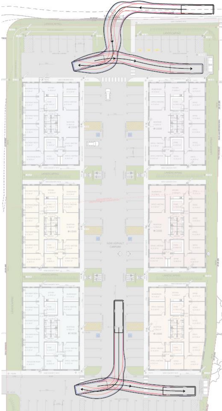
Figure 6 Swept path assessment – 10 m Rear-Lift Garbage Truck
