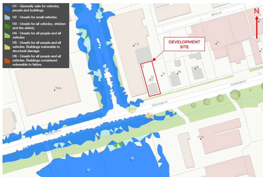
Figure 4 – Launceston City Council 1% AEP Urban (Stormwater) Flooding Maps
