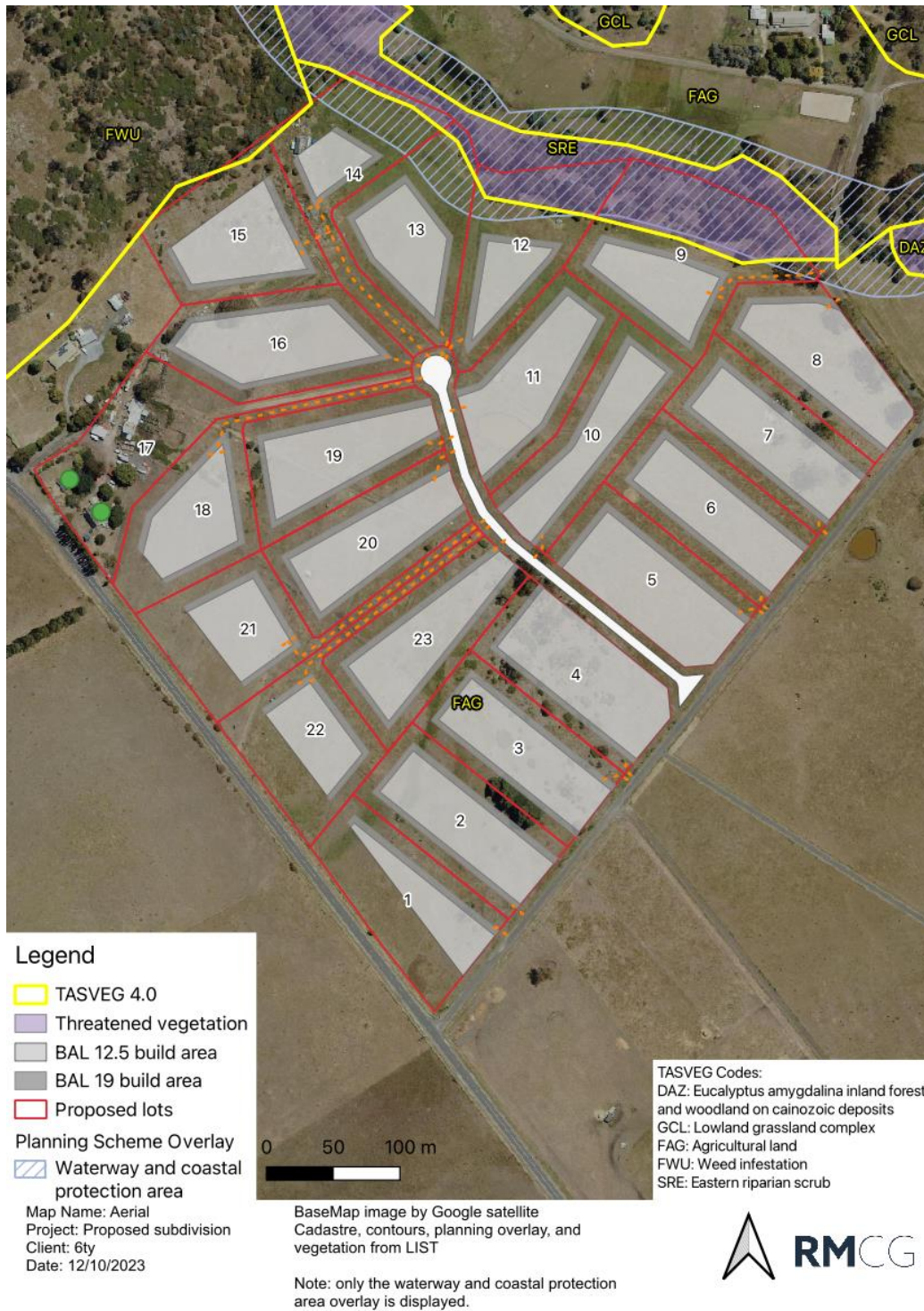
Figure A2-3: Proposal. Note access of Lot 9 passes through the waterway and coastal protection area (WCPA). Build areas and designed to avoid any impact on the WCPA and threatened vegetation, including when taking into account the required bushfire hazard management areas.
