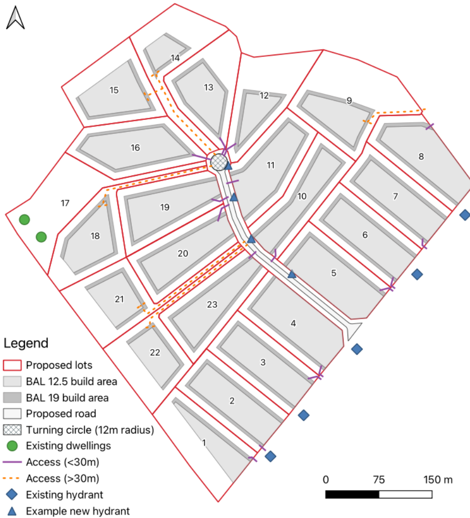
Figure 4-3: Access requirements and hydrant locations. Note, lot access and new hydrant locations area example only.
