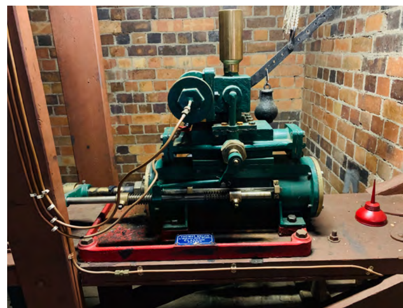
Organ Motor Room - hydraulic engine, made by Thomas Melvin & Sons, St. Rollox Iron Works, Glasgow Patent (inscribed on plate)
