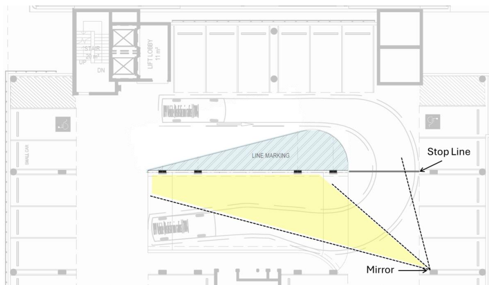
Figure 6 Level 2 ramp manoeuvring and visibility mitigations
