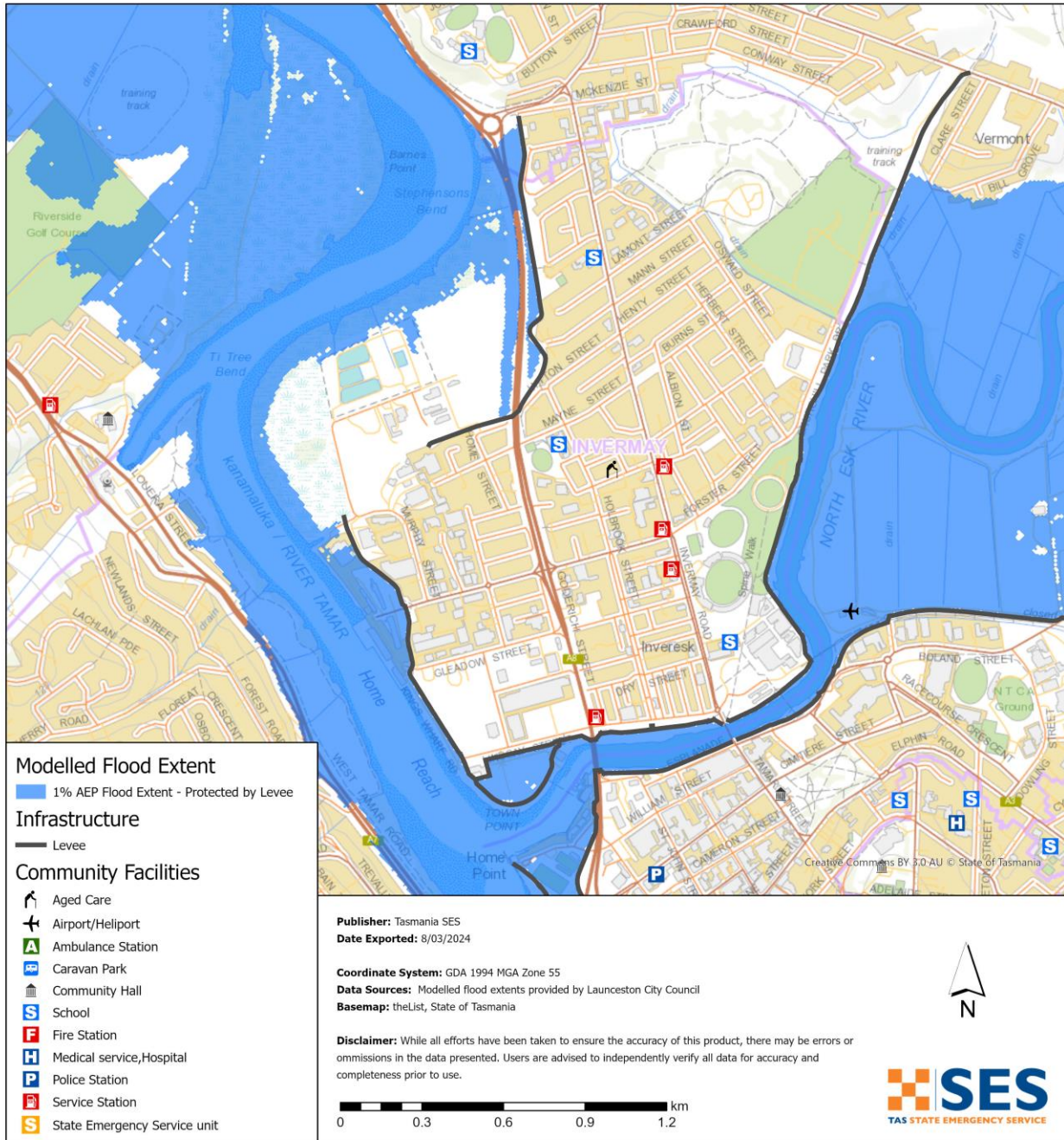
Map 1 – Levee Protected area of Invermay to a 1% Annual Exceedance Probability (AEP) flood event (Major Flood).
